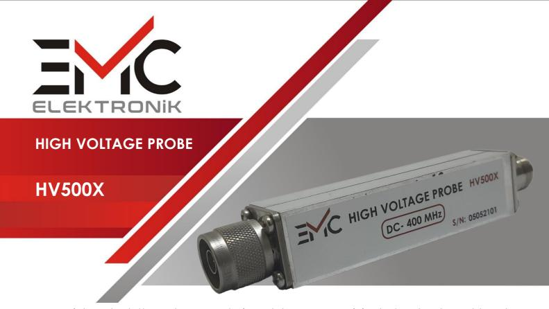
HV coaxial probe/attenuator was designed to measure injected pulse to cable when performing CS115 and CS116 calibration according to MIL STD 461. It has 500x voltage divider ratio. Its usable bandwidth is 400 MHz.
